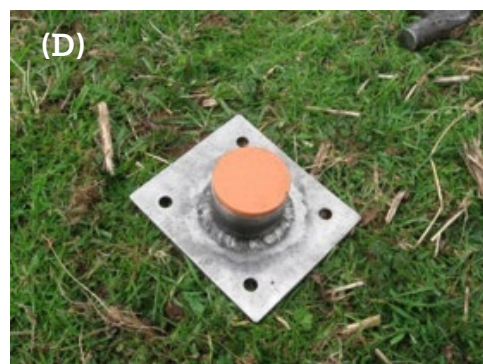
Figure 7: Geomorphic monitoring techniques used in the Bowmont valley. (A) an Unmanned Aerial Vehicle (UAV) used to survey the the river corridor at Swindon Haugh in May 2013, (B) topographical survey of a cross section of the Bowmont Water at Yetholm Mains in February 2012, (C) painted stone tracers in position in the Cocklawfoot Burn in October 2014 and (D) sediment impact sensor before installation on the bed of the Cocklawfoot Burn close to the gauging station.
