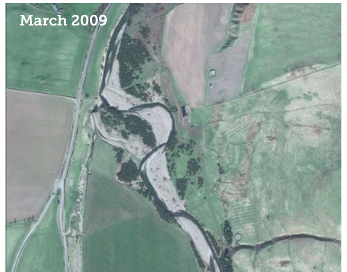
Figure 2: In response to the September 2008 flood, parts of the Bowmont Water experienced marked gravel deposition and changes in channel planform. Images show the Bowmont Water downstream of Attonburn (Imagery from Google Earth).
