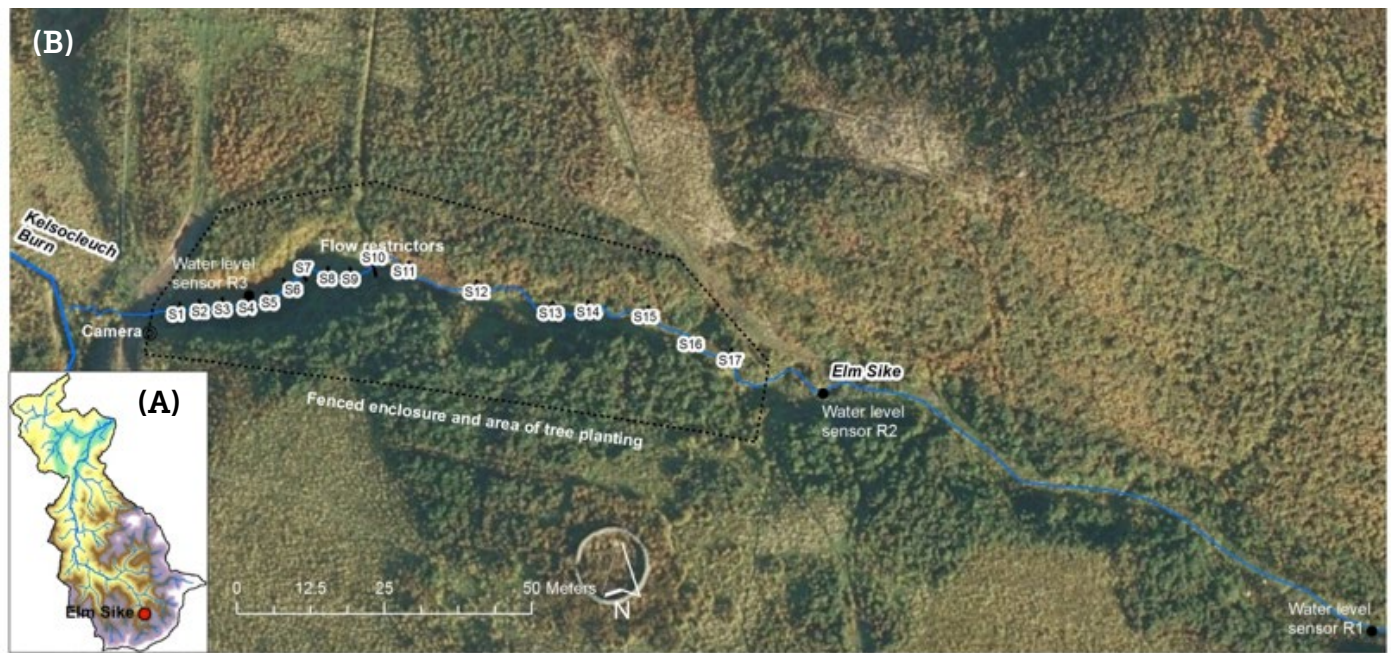
Figure 32: (A) Location of the Elm Sike study site. (B) Distribution of flow restrictors (S1 to S16) and water level sensors at the Elm Sike study site. Aerial photo dated to 2007 (Copyright Getmapping plc.).
