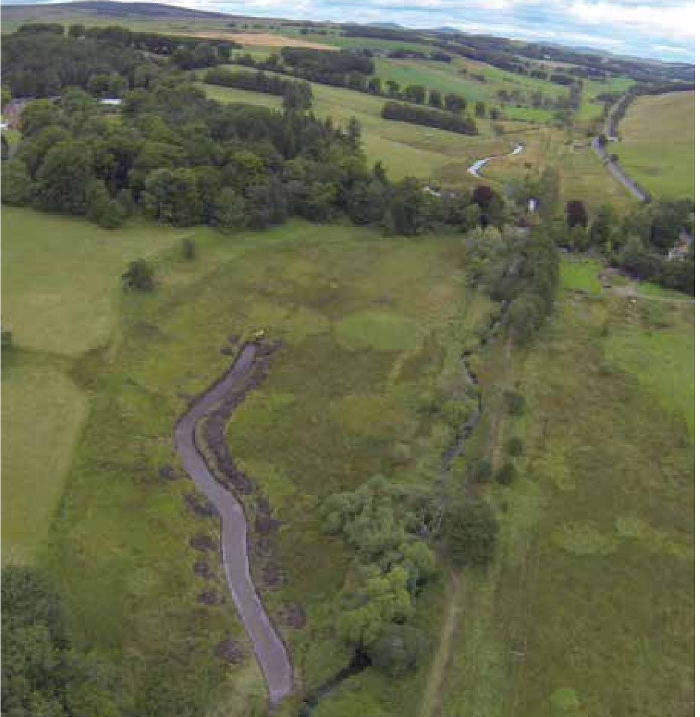
Figure 6.1. Remendering works taking place on the Eddleston Water, Scottish Borders (© Tweed Forum).
