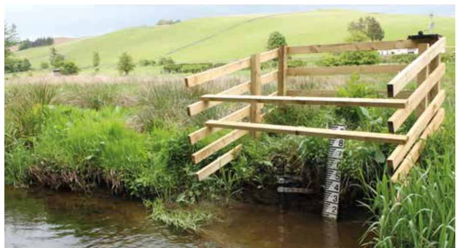
Figure 9.5. Gauging station level recorder on the Eddleston Water, Scottish Borders (© C. Spray).
