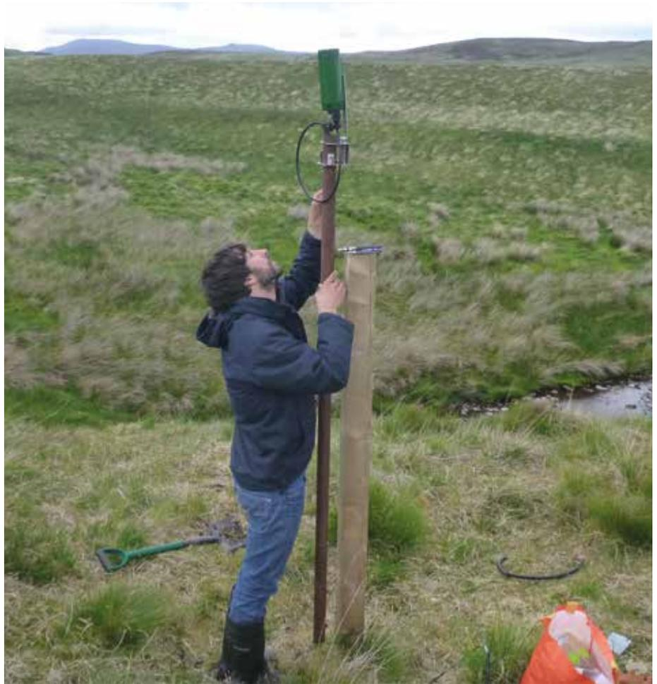
**Figure 9.6.** Installing a telemetered water level monitoring station in the Allan Water catchment (Forth), Stirlingshire: This station was installed to collect baseline data prior to woodland planting (© L. Bellini).
