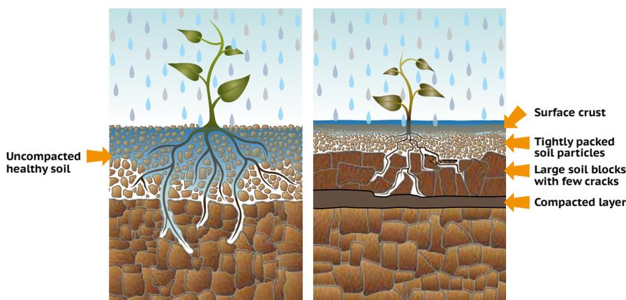
**Figure 2.3. Good soil structure (left) and compacted soil structure (right): Very little surface runoff is able to infiltrate into the subsoil layers due to the surface crust and compacted soil layers while vegetation is deprived of oxygen due to the compression of pores that normally transport air and water.**
