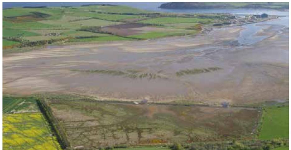
**Figure 3.10. Managed realignment at Nigg Bay on the Cromarty Firth, Ross and Cromarty. Two 20m wide breaches in existing sea defences were made to allow sea water to flood a 25ha field thus reducing the maintenance requirements of the existing failing defences and creating important habitat (© N. Russell, RSPB).**
