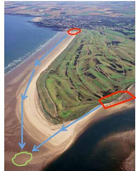
**Figure 10.14. Sediment pathways at West Sands: Areas of erosion are marked in red, sediment pathways in blue and areas of accretion in green – sediment was 'borrowed' and returned to areas of erosion.**
